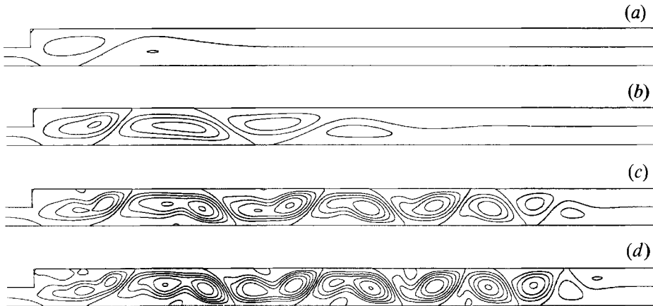
FIGURE 7. Effect of variation in the Reynolds number. Streamlines for St = 0.006 , e = 1 , t = 0.5 , -1.5 \leq x \leq 33.5 ; (a) Re = 125 , (b) Re = 250 , (c) Re = 500 , (d) Re = 750 .
